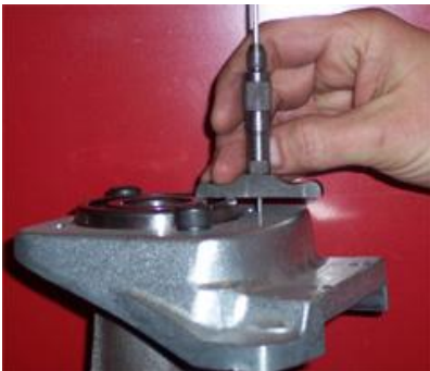
Figure # 2 – Installed Bearing Height
